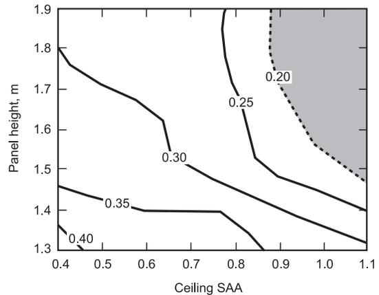
Figure 4. Shaded area shows combinations of workstation panel height and ceiling absorption (SAA) that can provide acceptable speech privacy corresponding to  $SII \leq 0.20$  for a 3 m by 3 m workstation.
