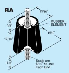
Mounts are designed for compression loading only. Standard mounts are not oil resistant.
