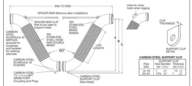
Drain Plugs are often removed to allow attachment of drain hose or steam trap for blow down or drainage.
